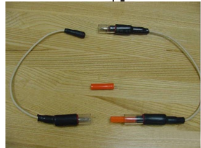
Figure 4: Fabricated jumper test leads.
