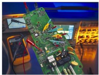
Minigrabbers and micrograbbers connect quickly to component test leads, terminals and integrated circuit leads. (Pomona models 5520, 5360, 4826)
