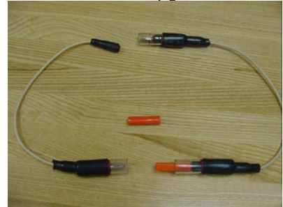
Figure 4: Fabricated jumper test leads.
